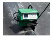
The hot wedge welding machine features integrated data recording and welding parameter monitoring. The myBAK-app guarantees quick access to data, and reports can be generated with just a few clicks.
