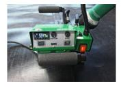
The small and light automatic welding machine to weld all different kind of materials. For civil engineering and tunnel construction. Combined wedge with hot air and contact. Location of the machine is known with the myBAK app.
