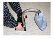
The reliable grooving machine to cut welding grooves into all different types of floor coverings without dust.
